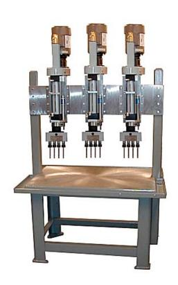
An AutoDrill designed Multiple Spindle Drilling Head system helped a customer fabricating doors to significantly increase their production drilling capabilities. The Multi-Drill fixture is capable of drilling all the hinge holes on a door in three separate hinge locations simultaneously. Multiple spindle drill heads and AutoDrill self-feeding drills reduce the multiple step operation to a single step.
