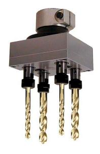
Close spaced holes tend to be uniform in size but there are situations where a hole pattern has hole sizes that differ. If the difference in hole size among the cluster of holes is less than 30-50% than the spindle speed can be set to allow drilling the largest hole size without affecting the tool life.
